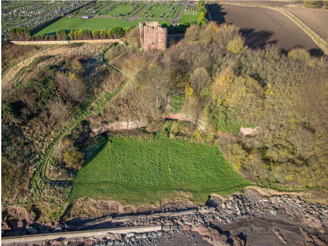
Illus 35: The upstanding portion of sea wall and broken concrete casing for the Rosie sewer pipe (Intervention 3, Table 5) and erosion bites behind it at Castle Green (Eddie Martin 2013).
